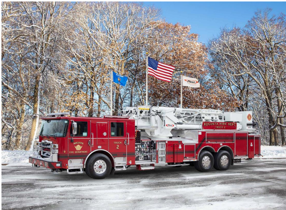
Pierce Enforcer mid-mount 100-foot tower ladder truck
