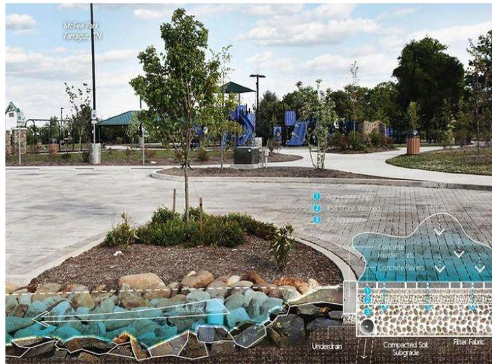
**Exhibit 4-3** Detail for Porous Concrete Pavers
