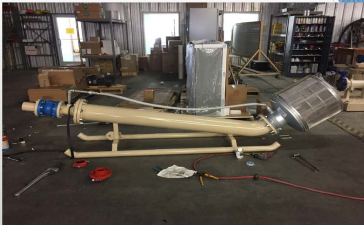
Suction Pipe with Self Cleaning Strainer
